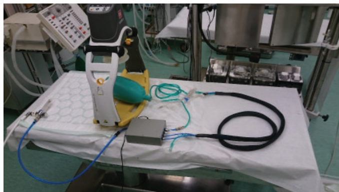
Our ventilator research prototype (gray box with tubing) together with the commercially available LUCAS chest compression device, developed at Igelösa.
